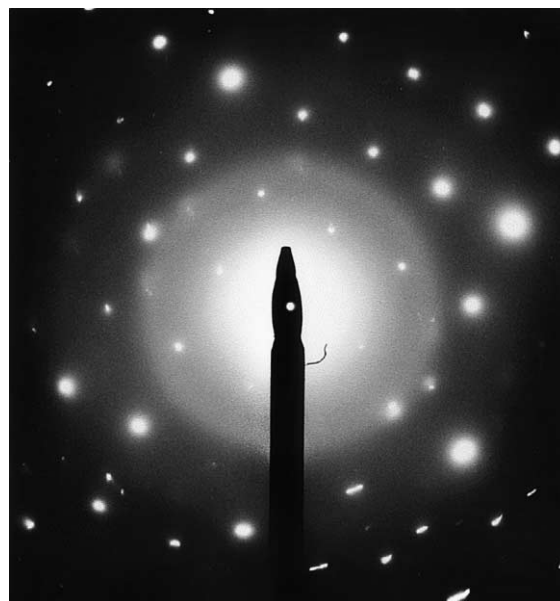
Fig. 1. Diffraction pattern after 2 \times 10^{13} Pb/cm ^2 implantation. The diffuse ring due to the electron diffraction on the amorphous zones and the diffraction maximum due to the crystalline remaining part are displayed.
